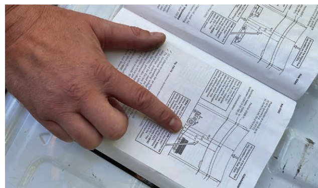
UP TO CODE: All line clearances must meet standards established by the National Electrical Safety Code. Clearances vary based on where the line spans.
