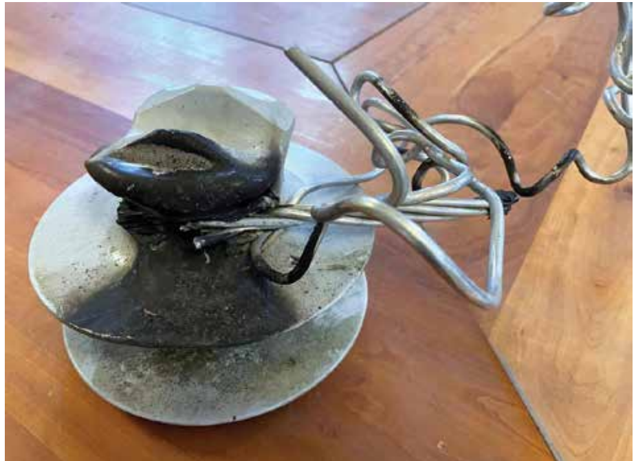
WHAT'S THE PROBLEM?: Blinking lights in homes and businesses can be caused by a wide range of issues, everything from animals and tree branches to equipment failure. Something as simple as a damaged insulator can take time to find and correct.
