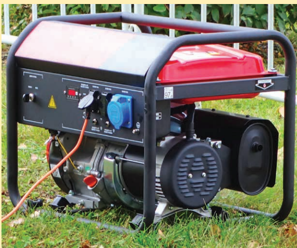
GENERATOR SAFETY: A portable generator sits outside in a well-ventilated area – a good safety practice!
